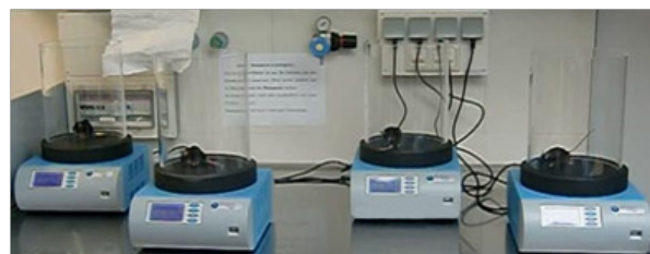
Fig. 2: "four Rotometers set up for high throughput screening, for testing several animals at the same time"
