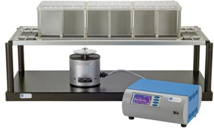
The **Dynamic Plantar Aesthesiometer (DPA)** was designed to automate the assessment of "touch sensitivity" and allodynia on the plantar surface of laboratory rodents and comes ready with all necessary accessories to work with both Mice and Rats. At each paw withdrawal, the DPA automatically detects and records latency time, and actual force at the time of paw withdrawal reflex.
