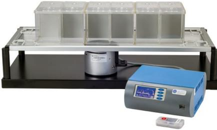
The **Plantar Test Instrument** (Hargreave's Method) measures the response to infrared heat stimulus, applied to the plantar surface. Our **Plantar Test** is the original apparatus, designed in close cooperation with Prof. Ken Hargreaves, who devised the method. Latency to paw withdrawal and infrared intensity are recorded automatically (i.e.no manual scoring, as in other models available on the market!).
